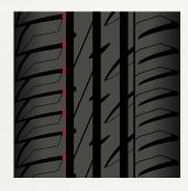
Low noise level Profile webs (so-called "Tie Bars") in the inner shoulder serve to reduce noise
