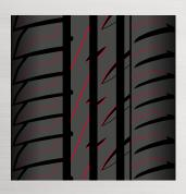
High wet grip for optimal handling and braking performance Sipes with multiple angles in the profile shoulders act like windscreen wipers when braking and the zigzag grooved indentations in the middle belts take out water and improve the handling in the wet
